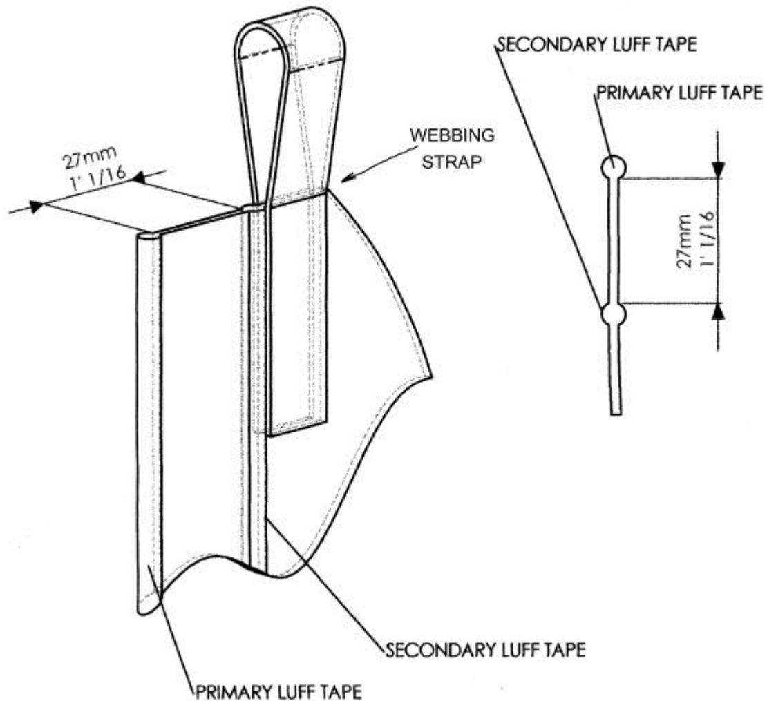
Adding a second luff tape as shown above will allow for clearing battens from feeder when hoisting or lowering sail at any point of sailing.
