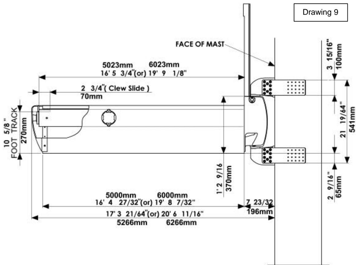
The PROFURL in-boom reefing system is delivered pre-assembled and in over-length. The boom profile (15) and the mandrel (16) will probably have to be re-cut to length to match the boat's requirements when fitting the system.
