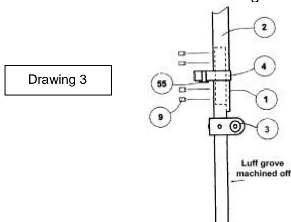
**III 4 b** - Completely insert a connector/articulation (4) at the upper end of the feeder profile (1) so that the Nylon bushing is turned towards the lower end of the feeder profile. Please see drawing 2 .
